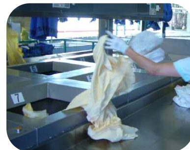
TAGSYS' SCH400 Smart Chute can be integrated at the soil sorting area
